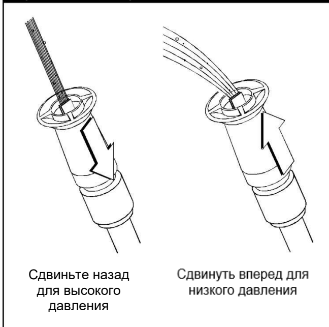
Figure 12 — Adjusting Nozzle for Pressure
